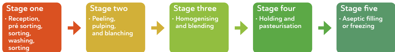
Figure 6. Production stages of sweet potato puree
