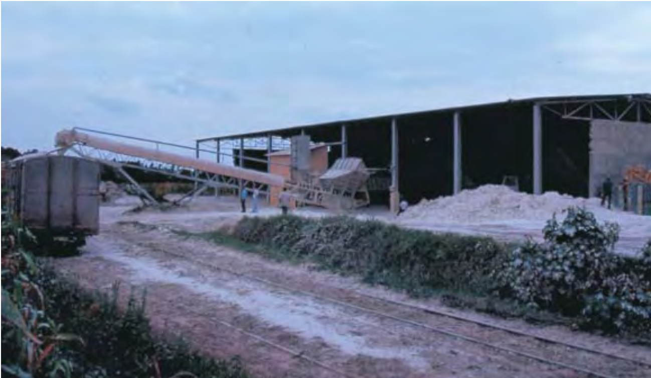
Figure Tanzania 9. Minjingu Mine, Storage Facility in Arusha at the Rail Line, 4000-Ton Capacity
