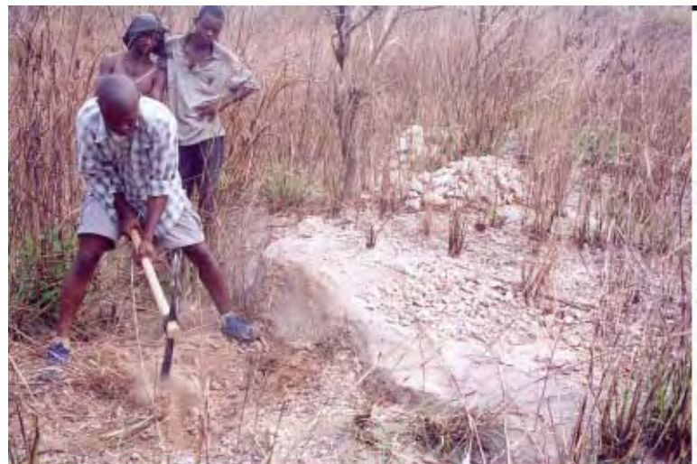
Figure Angola 8. Mondo Tando Deposit, Collecting Phosphate Rock Samples From Outcrop
