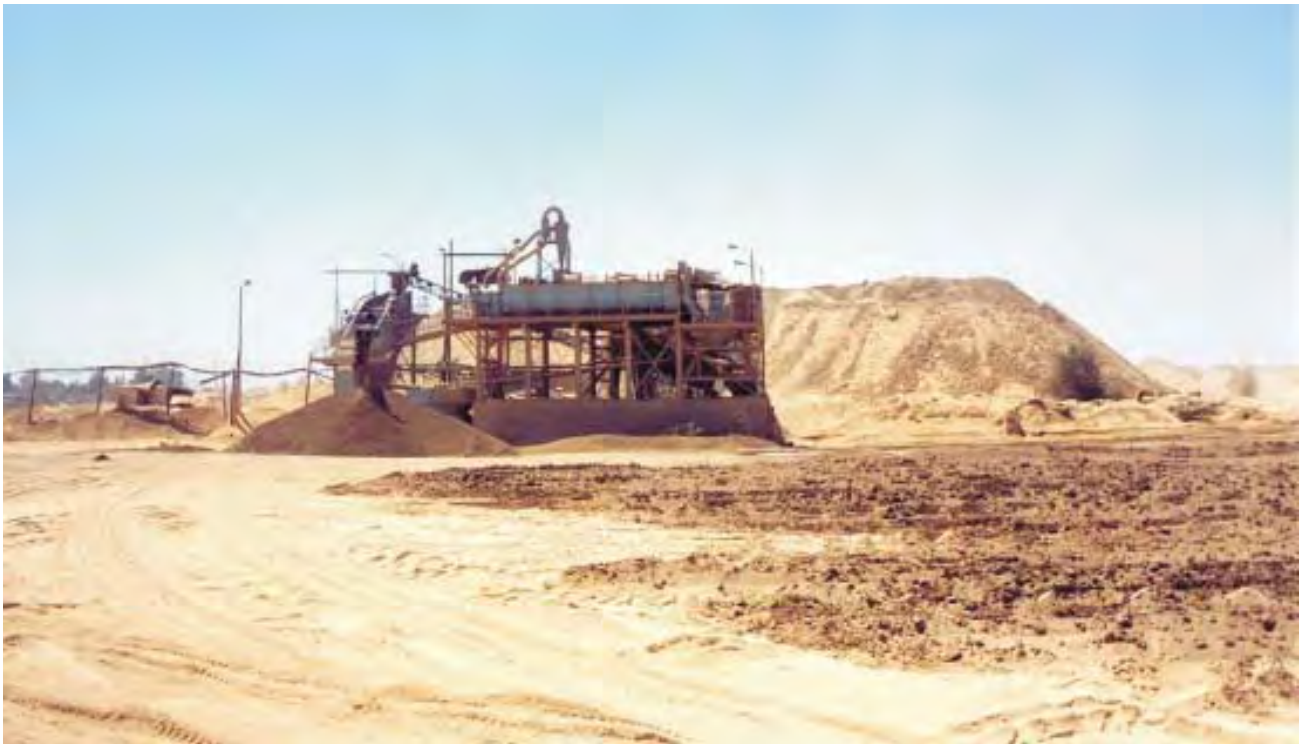
Figure Egypt 6. West Sebaiya Area, Crushing and Grinding Unit (Note Phosphate Rock Sun Drying in the Foreground)
