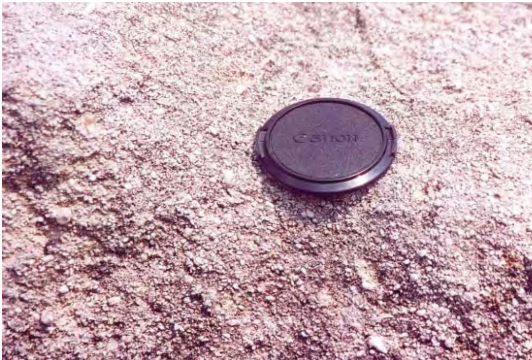
Figure Angola 10. Mondo Tando Deposit, Weathered Surface of Outcropping Phosphate Rock Showing the Coarse Granular Texture of Many of the Beds of the Cabinda Deposits
