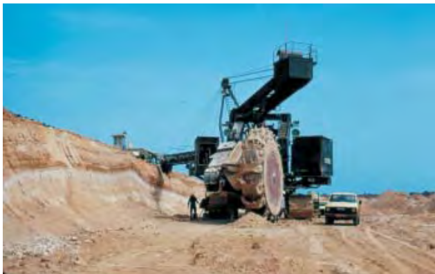
Figure Togo 5. Kpogame Mine, Togo, Bucket-Wheel Excavator Used to Mine the Ore Zone
