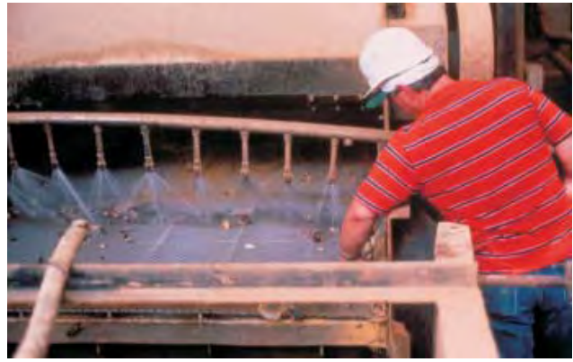
Figure Togo 9. Togo Beneficiation Plant, Initial Screening Station
